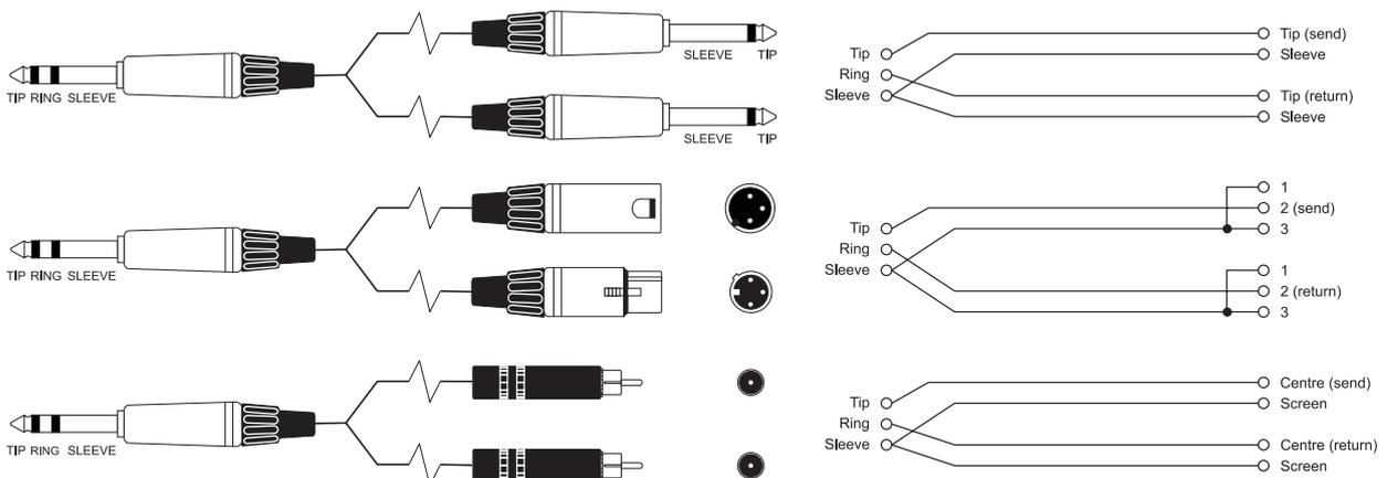
**'Y' Cables (Balanced)** Where used ... Aux, Mix outputs
