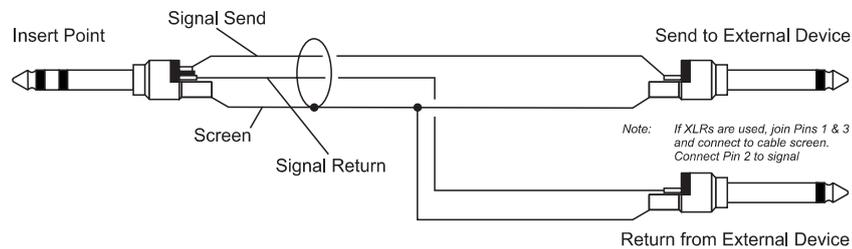
The Send may also be tapped off as an alternative pre-fade, pre-EQ direct output if required, using a lead with tip and ring shorted together so that the signal path is not interrupted (see below).
