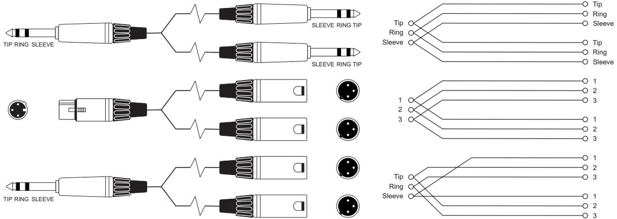
**Headphone Separator** Note: for every doubling of headphones the load impedance is halved. Do not go below 32 Ohms.
