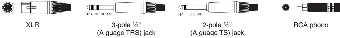
Balanced - Line Inputs, Mix L & R Outputs, Stereo Inputs, Auxiliary Outputs
