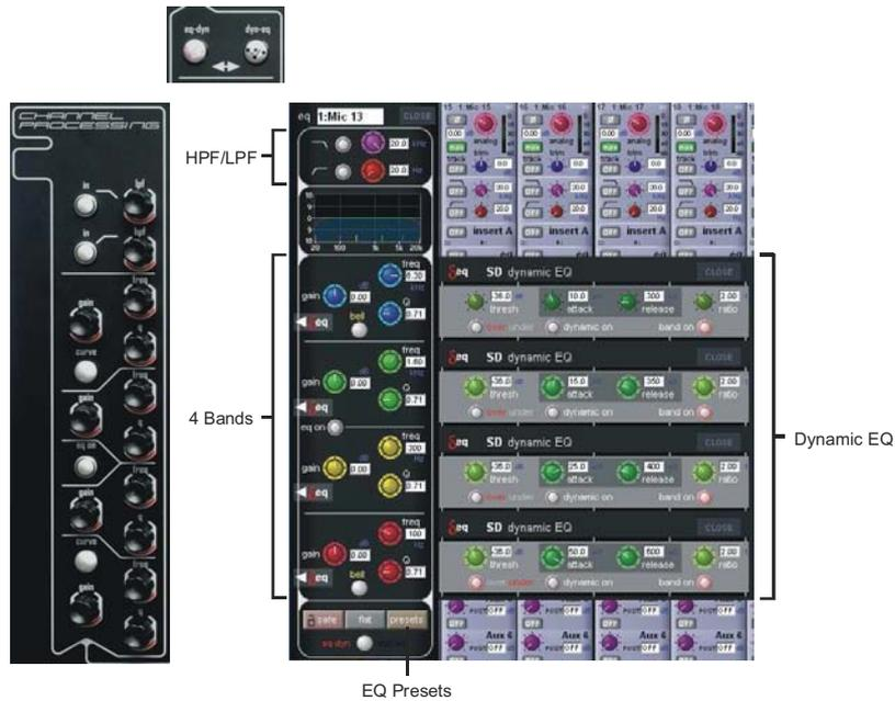
In both the EQ/filters display and on the worksurface, each band has a  $\pm 18$ dB gain controller on the left, a frequency controller (ranging from 20Hz to 20kHz) top right and a Q control bottom right. Each pot has its value displayed to its right. The top and bottom EQ bands have **Curve** buttons that allow the filter type to be switched.
