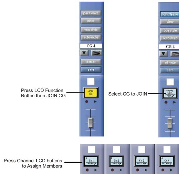
2) Press the on screen JOIN/LEAVE button for the required CG channel
