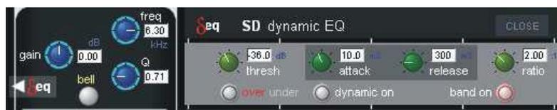
To place the dynamic module into Over mode, ensure that the Over indication below the threshold control is not illuminated.
