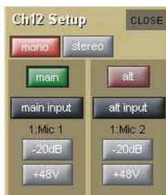
The inputs available on an Input channel include feeds from the external IO racks, the local inputs on the back of the console and a variety of internal signals. Pressing either the **main input** or **alt input** routing button in the **Setup** display opens the **Input Route** display. The signal feeding each input can then be selected as described in the Getting Started section of this manual.
