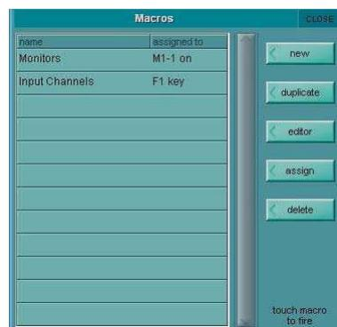
This is where macro commands can be assigned to the 8 buttons in the **macros** area located in the left hand section of the console (shown below), as well as to the function (F) buttons on the external keyboard and to the console's GPIs. Macros can also be fired directly from this list by touching the macro when none of the right-hand buttons is active.
