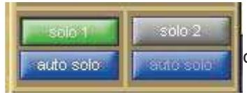
The channel's solo routing is assigned in the section at the bottom section of the channel Setup display. Pressing the green **solo 1** and **solo 2** buttons enables the channel to be routed to solo busses 1 and 2 respectively. The buttons are green to indicate that the solo bus is available, and grey to indicate that it isn't.
