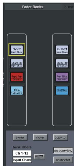
To swap the locations of two fader banks, touch one bank button so that it is highlighted in yellow, touch **swap** (located below the left fader bank's) and touch the other bank button.
