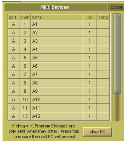
The SD9's built in MIDI port is referred to as Port A in the **Port** column.
