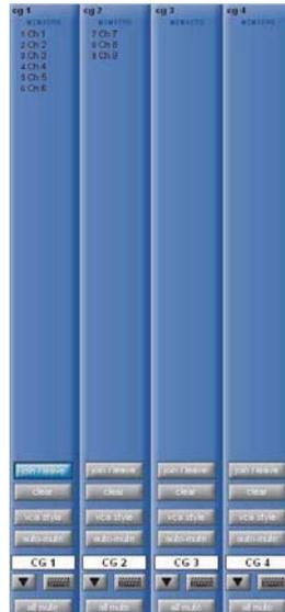
**Note that Control Group channels function completely differently from Group (GRP) channels: Group channels mix together the audio from any channels routed to them, whereas Control Groups simply allow adjustment of the levels of the channels to which are assigned to them, irrespective of any audio routing.**
