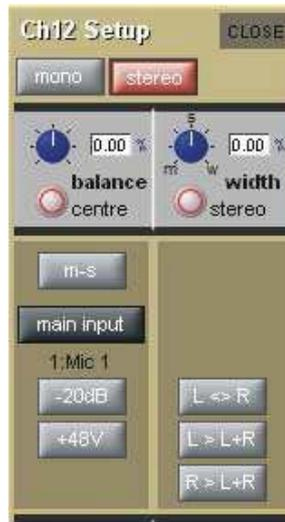
Stereo channels also have an **m-s** button, located above the input routing button, which switches in a decode function for replaying M-S signals as a normal stereo pair. There are three further buttons in this panel: **L<>R** swaps the channel's left and right outputs, **L>L+R** sends the left signal to both left and right busses, and **R>L+R** sends the right signal to both left and right busses.
