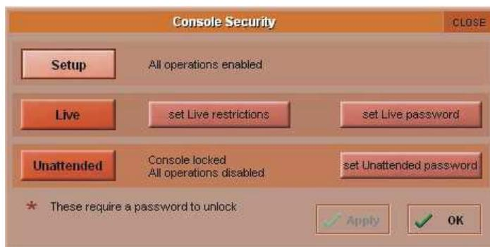
User passwords can be defined for the Live and Unattended modes. To set a password, press the Set Password button. Enter the old password, then enter the new password twice.
