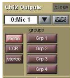
Any mono groups being fed by a stereo channel will receive a L+R summed signal of the channel output.
