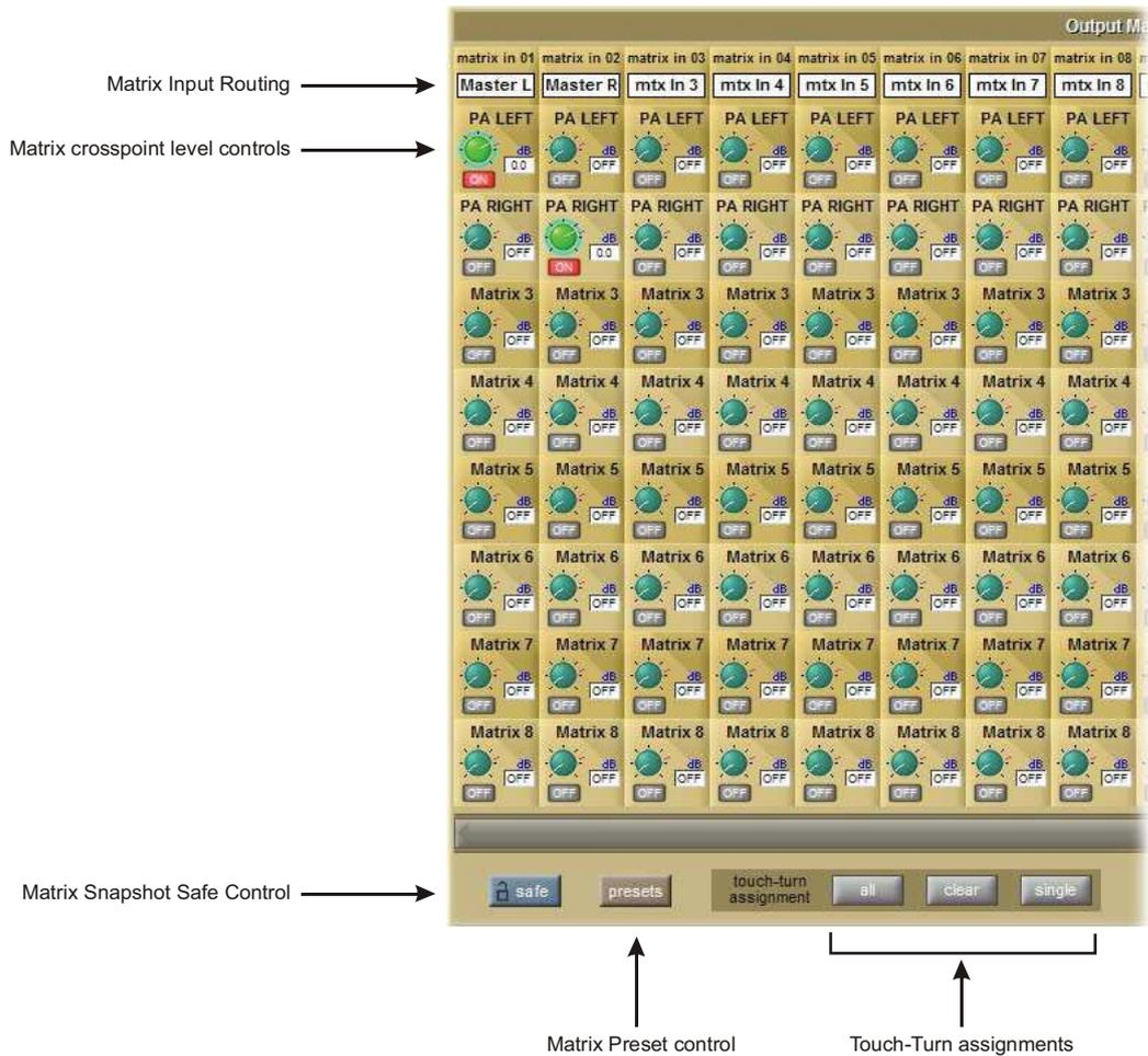
Each pot within the display trims the signal coming from the input for that column, going to the output for that row. The top of each input column displays the input's name, and the label above each trim pot displays the pot's matrix output. Touching any trim pot assigns it to the Touch-Turn encoder, and the pots lighten and are ringed green to indicate that they have been assigned.
