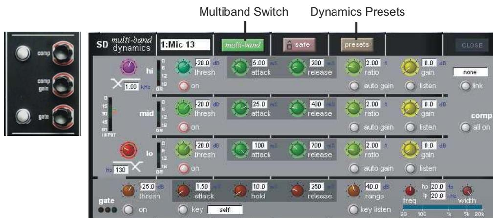
Up to 4 Channels can have their Dynamics (Compressor) modules switched into Multi-band mode
