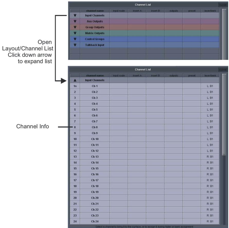
Primarily, the **Channel List** display is used for adjusting the bank assignments of the session's channels. This function employs the **COPY BANK FROM** LCD function mode, and is described in full in the Channel Types section of this manual.
