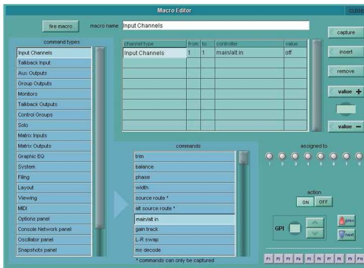
The name of the macro being edited is shown at the top of the display. To switch to a different macro in the list, touch the new macro in the Macro display list (You may need to move the displays around the panel to access the list). To rename the macro, touch the **macro name** text box, type the new name in the on-screen or external keyboard, and touch **OK** - This name will be used in the Macros display.
