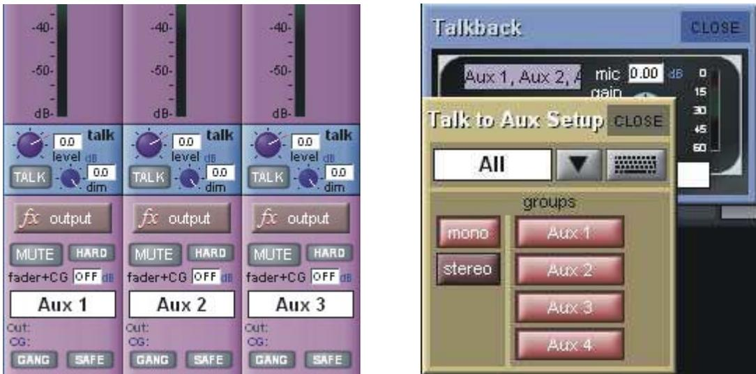
On the Aux Output channels, press **Quick Select Aux** and the row of assignable controls beneath the screen can be used to switch Talk to Aux On/Off, control the level of talkback signal and set the level of dim when the talk is active. This **Dim** level setting is a 2nd Function so press the 2nd Function button and use the under screen control to adjust it.
