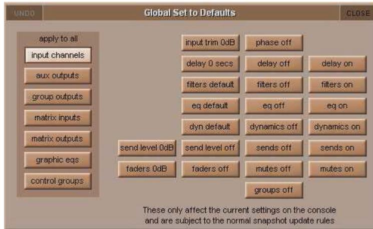
The Global Set to Defaults Panel allows global settings to be applied to the console. Open the Global Set to Defaults Panel from the Files Menu. Select the Channel type from the list on the left side of the panel, and then select the operation to perform from the available functions. An undo function is provided which undoes all changes since the panel was opened. Once the Global Default Panel is closed, changes cannot be undone.
