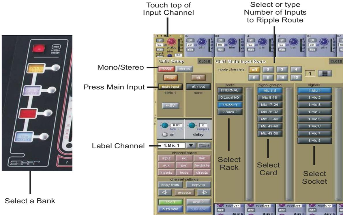
Within each display, there are three columns containing three levels of routing selection:
