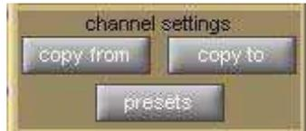
The **copy from** button allows settings to be copied from other channels to this channel and those to its right: Pressing **copy from** opens up a **Copy Channels** display:
