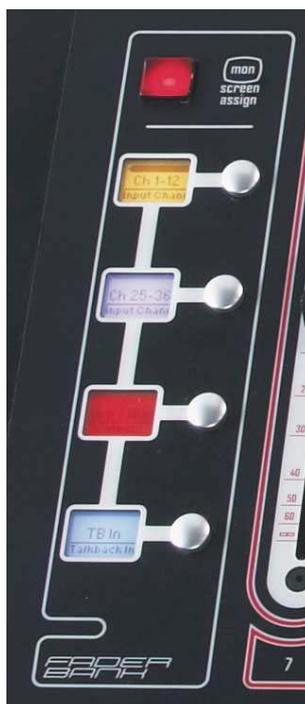
A 'bank' is a set of twelve faders, and a "section" contains up to four 'banks'. There are two sections of the desk, allowing up to 96 channels to be accessible on the worksurface.
