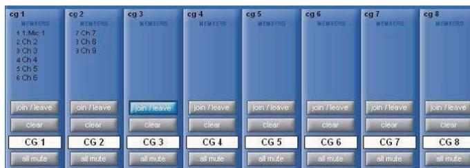
This display consists of basic versions of each Control Group channel strip, including the channel assignments lists and a number of basic settings which can also be adjusted in the display: **join/leave**, **clear** and **all mute**. The Control Group naming controls are also available within the display's channel strips.
