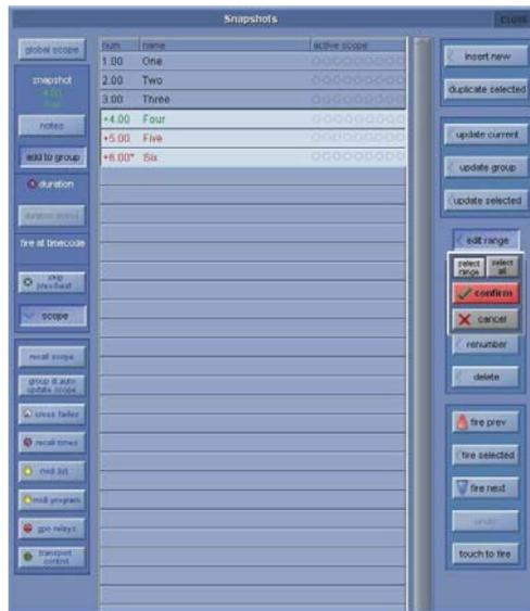
With the Edit button pressed, pressing the Snapshot buttons does not fire the snapshots, it only selects them for editing. The selection may be changed by pressing and releasing snapshot buttons at any time during the operation of the Edit command, so a variety of controllers or routes may be changed in a variety of snapshots before completing the operation by pressing the **Confirm** button.
