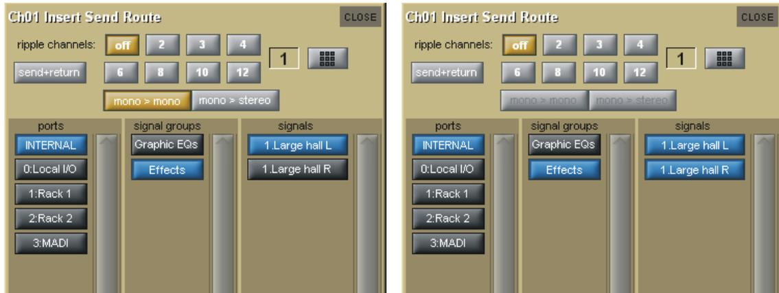
When routing to Internal FX using an auxiliary, the FX send is also configured according to the channel type (Mono or Stereo) but a Mono auxiliary can be set to provide a stereo FX output by pressing the **Mono>Stereo** button and rerouting.
