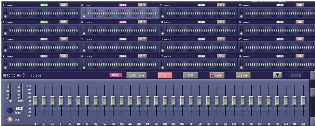
The settings on each graphic EQ are accessed via the expanded display, though some settings can also be adjusted in the miniature display. Touch any of the graphic EQs to assign it to the expanded display. Touch an area of the expanded display to assign the Graphic EQ faders to the 24 worksurface faders on the console.
