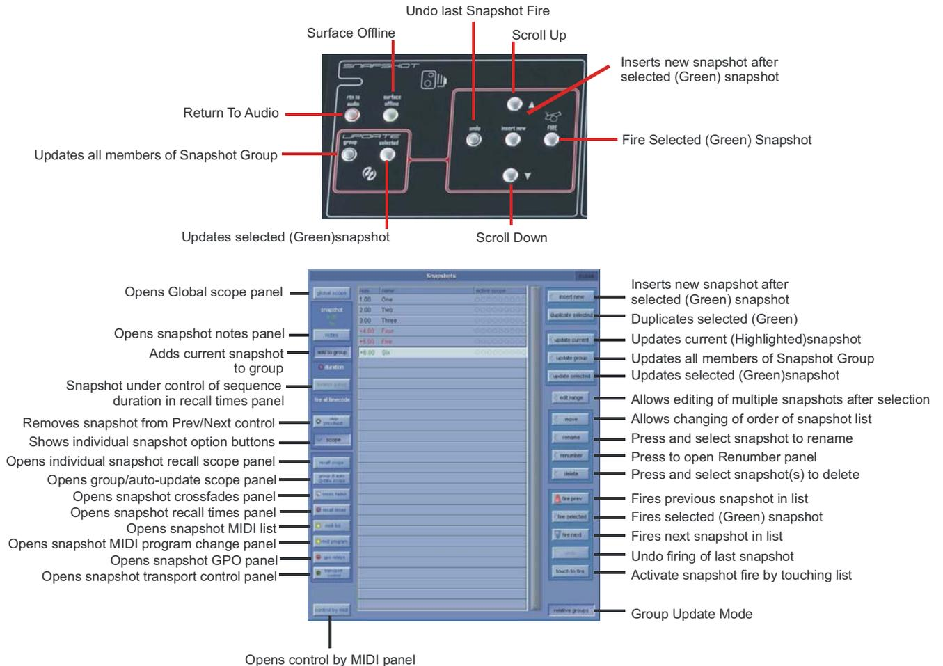
**Note - The current snapshot appears in the panel as the highlighted (pressed) button. The snapshot name displayed in green indicates that it is the selected snapshot. The Fire button recalls this selected snapshot and highlights it in the screen list as the current snapshot.**
