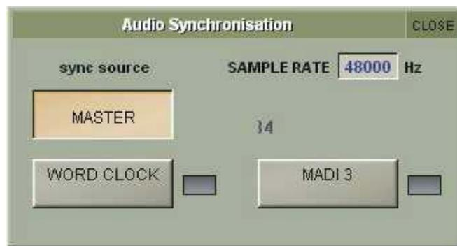
The SD9 will operate at a sample rate of 48000Hz (48kHz), and the current rate is indicated in the **SAMPLERATE** box at the top of the display.
