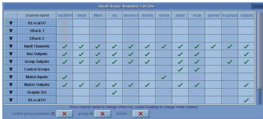
This is very similar to the Global Scope panel but represents the Recall Scope for one individual snapshot which is indicated by its name and number at the top of the panel.
