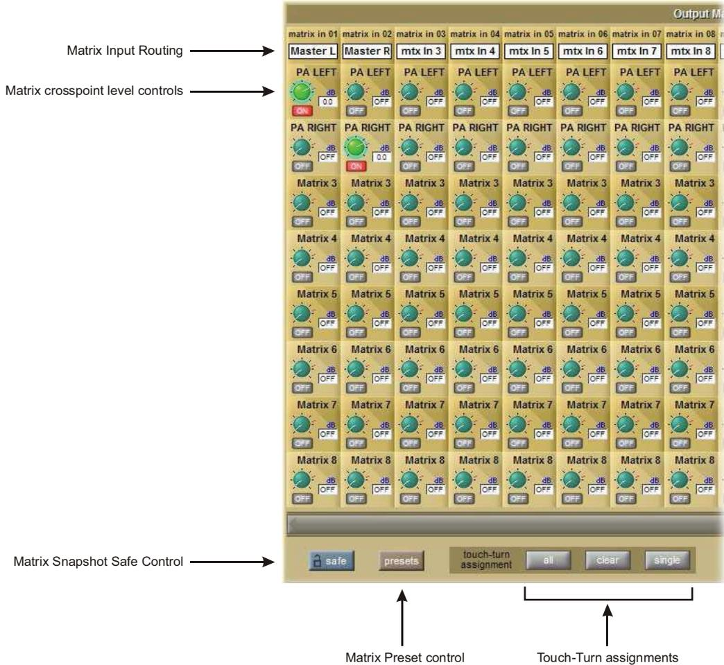
The example above has the Master Stereo Buss routed to the inputs of Matrix 1 and Matrix 2 (Labelled as PA LEFT & PA RIGHT). By adjusting the crosspoint levels, you can change how much of each side of the Master buss is fed to these Matrix Channels.
