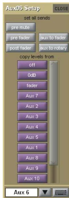
The grey **set all sends** buttons at the top of the **Setup** display affect the sends to that aux bus from all of the Input channels. The three buttons on the left, **pre mute**, **pre fader** and **post fader**, set the point in the channel from which the aux send is taken. The current send point is displayed next to the aux send level in the Input channels.
