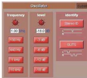
The frequency of the oscillator is controlled by the left-hand **frequency** pot, and its audio level is controlled by the right-hand **level** pot. The buttons below each pot, can be used to set the oscillator to standard frequencies (**100Hz, 440Hz, 1kHz, 10kHz**) and levels (**-3dB, -6dB, -12dB, -18dB**). The current value of each parameter is displayed below its pot.
